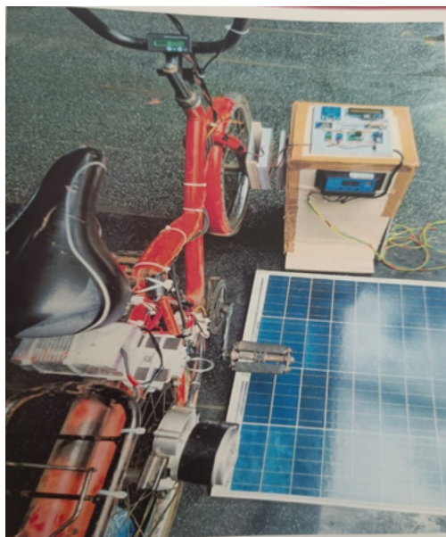
Figure 7.5.4: Solar powered wireless charging station for E bicycle with IoT
