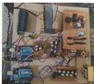
Figure 7.5.9: Remotely Located energy meter monitoring with load control and mobile billing system
