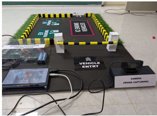
Figure 7.5.12: Automated boom barrier control with intelligent Image processing for vehicle management
